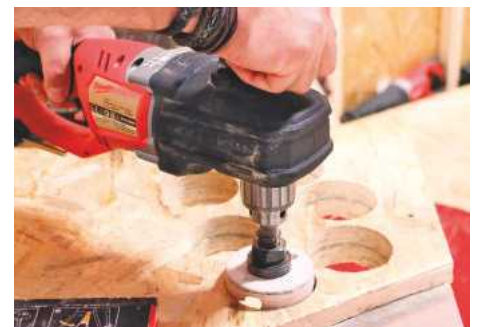
▲ Switching to a holesaw allows you to cut bigger diameters through steel as well as wood
